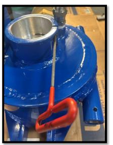
5. Remove the gearbox from the job box and inspect for any damage or binding. Check internal bore for any debris and clean if necessary.
