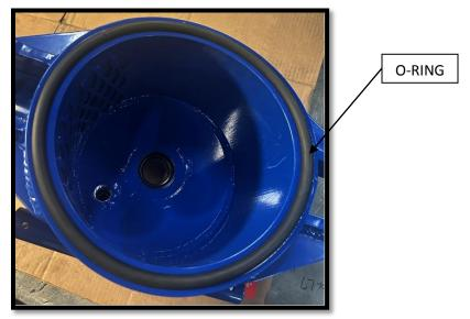
3. Place on the flat surface to begin assembly – be sure this is placed with the O-ring side down. Put rags or a welding pad down under the housing to avoid getting dirt or debris on the O-ring.
