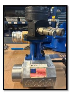
13. Rotate motor as shown once the set screws have been tightened and install the supplied %"-13 x 2" Socket Head Cap Screws and Hex nuts.
