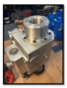
9. Install the hydraulic motor drive coupler onto the shaft of the gear box. Use supplied allen wrench to tighten set screws retaining the coupler on the shaft.
