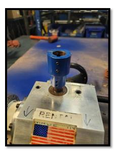
11. Install hydraulic motor adapter housing onto the side of the gear box. Install 3/8"- 16 X 1 1/8" Socket Head Cap Screws. Set screws on the drive coupler should be accessible through the slot in the adapter. Tighten the screws with the supplied allen wrench.
