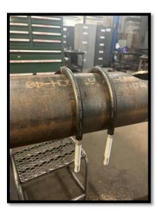
2. Using the handles on the Modu-Tap system, two people are required to position the housing under the section of pipe.
