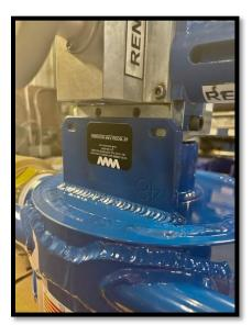
17. Install the retainer clip as shown with the supplied  $\frac{1}{4}$ "-20 Socket Head Cap Screws. Tighten socket head cap screws on the retaining collar until snug.
