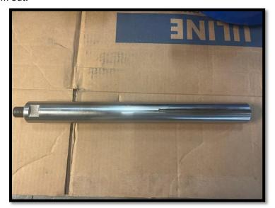
15. Lubricate the inside seal of the Modu-Tap housing with WD40. Install the boring bar into the gear box to check the alignment of the keyway. If misaligned, the boring bar will not slide easily into the gearbox. If this occurs, loosen the mounting bolts and allow the boring bar to center the adapter on the gear box opening and tighten down the adapter mounting bolts.
