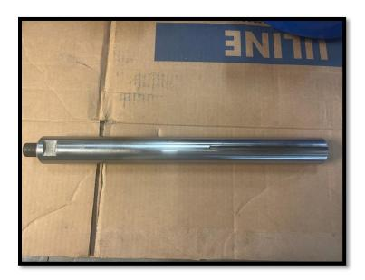
15. Lubricate the inside seal of the Modu-Tap housing with WD40. Install the boring bar into the housing to check the alignment of the keyway, gearbox and housing. If misaligned, the boring bar will not slide easily into the gearbox. If this occurs, loosen the mounting bolts and allow the boring bar to center the adapter on the gear box opening and tighten down the adapter mounting bolts.
