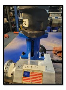
13. Rotate motor as shown once the set screws have been tightened and install the supplied  $\frac{13}{2}$ "-13 x 2" Socket Head Cap Screws and Hex nuts.
