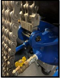
Flat lip section of hook block will be visible when pin is fully seated.
