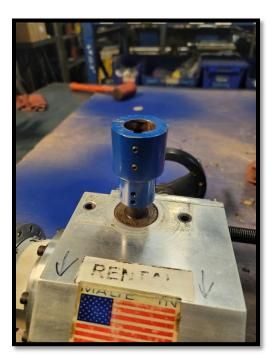
11. Install hydraulic motor adapter housing onto the side of the gear box. Install 3/8"- 16 X 1 1/8" Socket Head Cap Screws. Set screws on the coupler should be accessible through the slot in the adapter. Tighten the screws with the supplied allen wrench.
