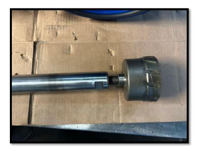
19. Apply cutter paste to carbide cutter, making sure some gets on each tooth. Use caution as the teeth of the cutter are very sharp.
