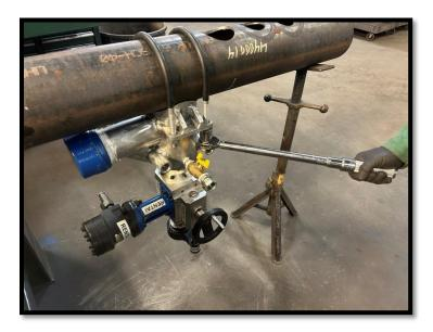
6. Check to ensure the housing is compressed against the pipe and you have an equal gap all the way around. Note: It is normal for the O-Ring to protrude a bit once the unit is torqued.
