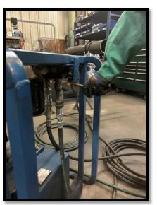
8. Slowly turn feeder handle, engaging the cutter into the pipe, apply constant light pressure to the feeder handle. Do not force the cutter into the pipe as this could stall the hydraulic power unit or damage the carbide cutter. Should the cutter stop turning, retract the cutter head by turning the feeder handle in the opposite direction. After the cutter is free slowly crank the handle to engage the cutter back into the pipe.
